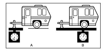
If a weight-carrying hitch or a weight-distributing hitch is being used, the trailer tongue (A) should weigh 10-15 percent of the total loaded trailer weight (B).
